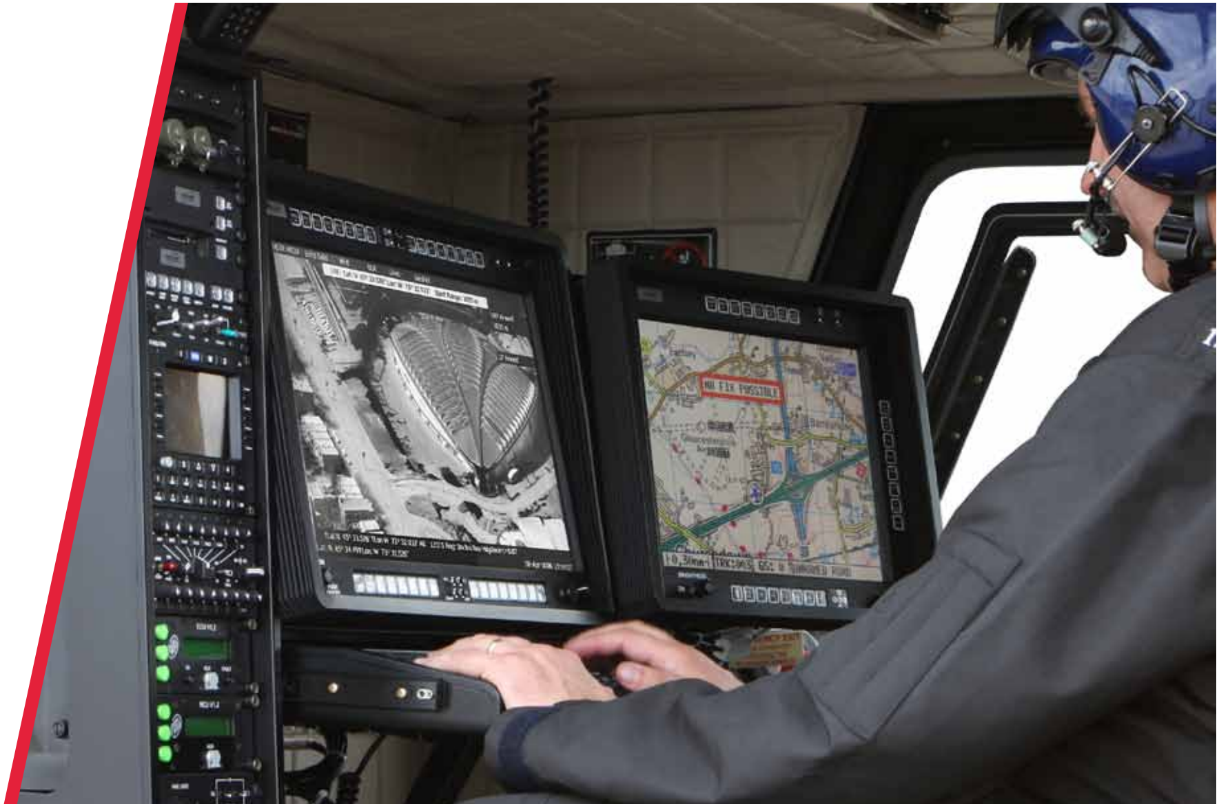
Rear mission console in MD902 helicopter used by Greater Manchester Police in the UK. Skyquest AVDU-5008 20" high-definition mission display (left) and AVDU-3824 15" display (right) along with integrated QWERTY keyboard with NVG backlighting.
