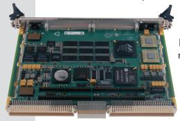
ne 183 satisfies the most demanding requirements of embedded computing applications. Available in the full Curtiss-Wright Controls Embedded Computing (CWCEC) range of environmental build grades the 183 is targeted to the sophisticated data- and digital signal-processing needs of tactical aircraft, armored vehicles and harsh environment naval systems.
