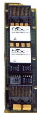
Figure 10: Interface Personality Module with MIL-STD-1553
