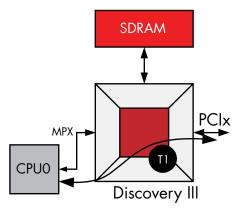
While transaction T1 is in process on the PCI bus, one or more transactions, Tn, to a faster target such as SDRAM can take place
