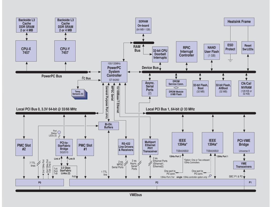
for transmission across the StarFabric network, supporting multiple routing methods including standard PCI addressing as well as path and multicast routing. StarFabric's scalable architecture allows engineers to design custom network topologies, connecting multiple bridges and switches together with unlimited flexibility.
