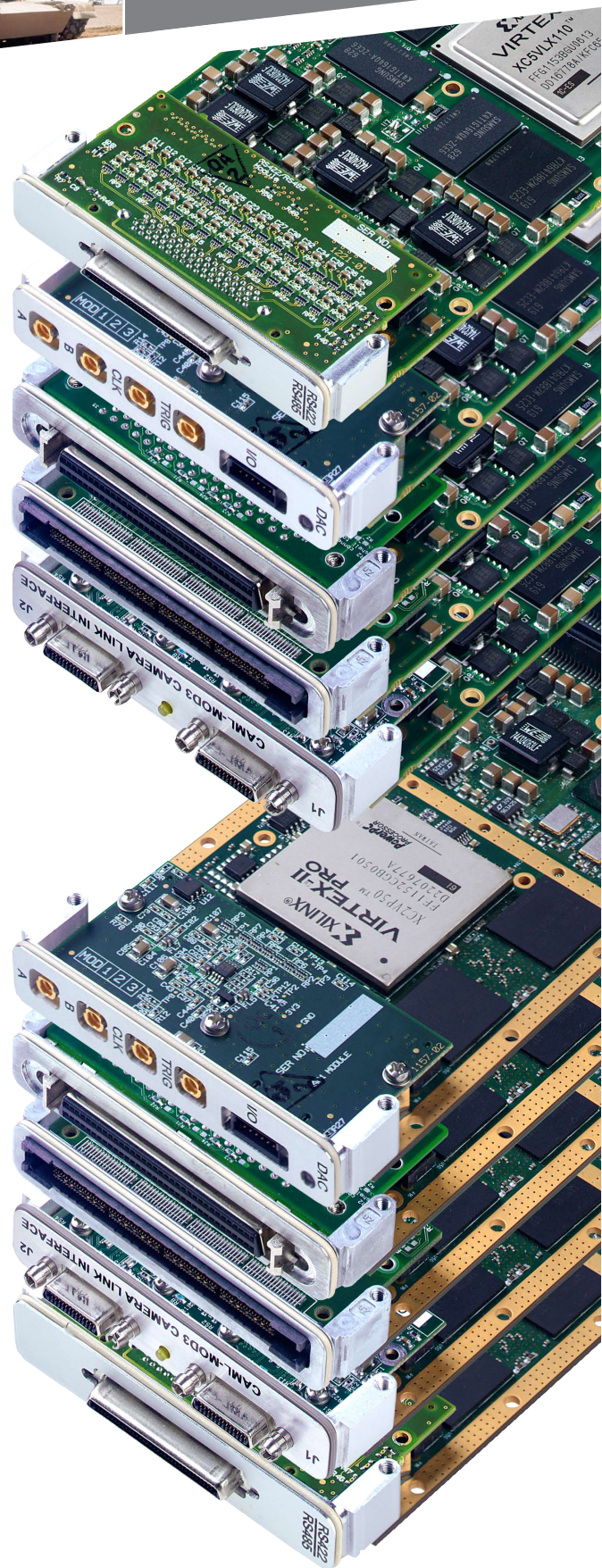
Figure 4: Modules fitted to Virtex-5 PMCs (above) Virtex-II Pro PMCs (below)
