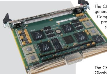
The CHAMP-AV IV is supported with operating systems including VxWorks, Linux, INTEGRITY and Gedae. Curtiss-Wright provides signal processing libraries and a high performance Inter-Processor Communications Library for message passing and bulk data transfers, which extends to multiboard systems utilizing StarFabric.
