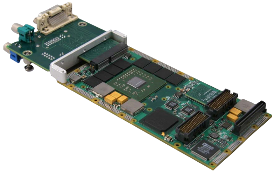
Figure 3: Photograph of an air-cooled XMC-710 (Variant with Front Transition Module)
