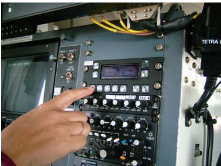
Figure 2: The optional remote control panel which can be used to control several recorders on the same aircraft.
