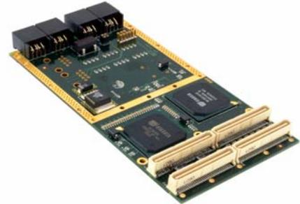
Many signal processing problems demand the use of multiple processors to achieve real-time throughput and response times. For applications of this type, it is invariably necessary to share large amounts of data between the processing nodes. The StarLink II PMC adaptor provides a modern technology solution to this problem with many specific benefits for the military aerospace systems designer.
