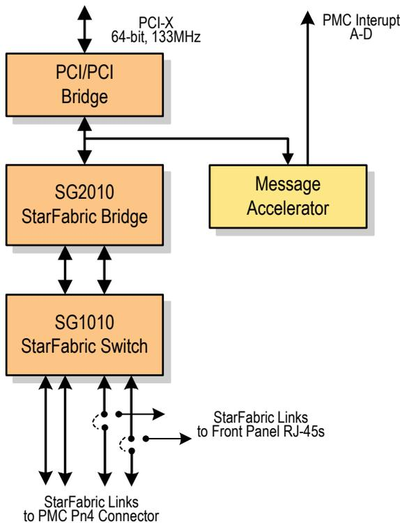
Figure 1: StarLink Block II Diagram
