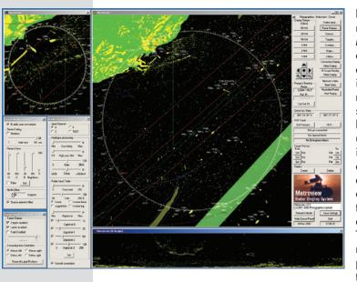
Primary radar video may be received by Metroview from either a local radar input card or from a network interface using a remote radar video server, such as Curtiss-Wright's RVP product. When used with a local radar input card, analogue or digital radar video and associated turning data are received by the system and transferred to a radar scan converter. The scan converter renders the radar pictures by transforming the incoming radar data
