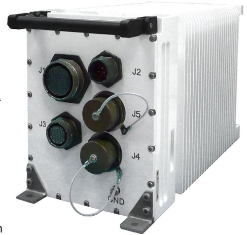
The MPMC-9341 uses advanced packaging techniques to provide the processing power of up to four single board computers (SBCs) in a rugged enclosure that measures a compact 600 cubic inches, yet is able to operate and survive external air temperatures of 55°C using only natural convection. This enables system designers to implement and deploy a highly capable processing system without the need for fans, coldplates, vehicle supplied air, liquid or other supplied resources.
