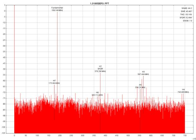
Figure 7: Channel B Signal Frequency: 1310.9MHz (aliased back to ~189MHz), Sample Frequency 1.5GSPS
