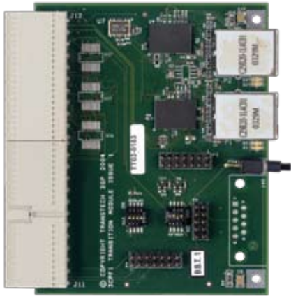
Figure 7: 3CPF1 Transition Module
